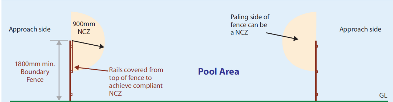
Boundary Fence Used as a Pool Barrier AS1926.1 - 2012
