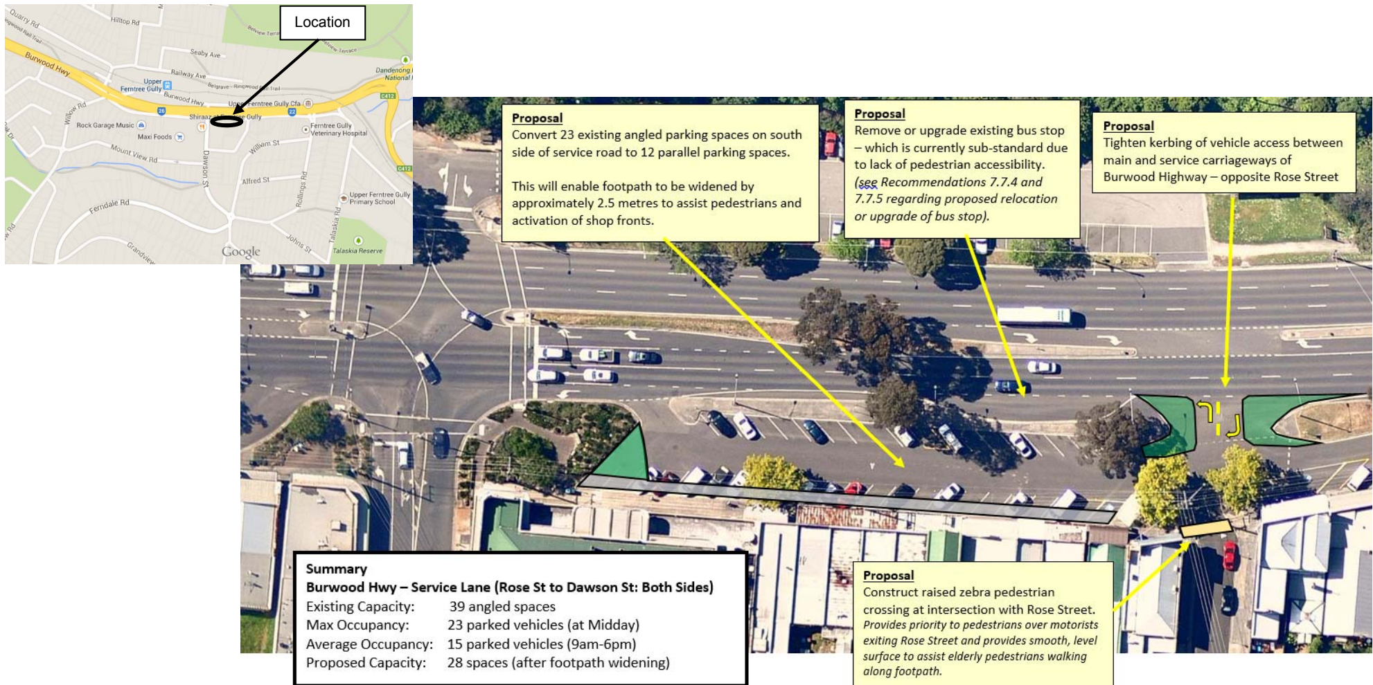
Figure 49: Burwood Highway Service Road – Rollings Road to Dawson Street
